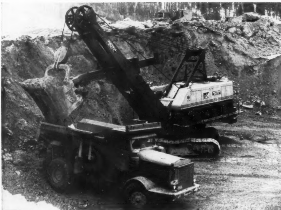
TRUCK-SHOVEL teams moved the blasted rock to expose the Craigmont ore body. Here a new Bucyrus-Erie 88-B Diesel shovel with a five yard bucket loads one of the 14 Euclid 27 ton Diesel trucks. Two 2½ cubic yard Northwest 80D shovels were also used for stripping. This is first rock cut and it shows mixture of soil, boulders, and blasted rock.
